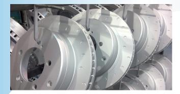
The addition of Zinc as a functional pigment in relatively high levels to an organic binder is one of the most important types of anti-corrosion protection sytems.
